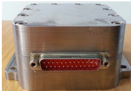
Figure 16. Medium-speed data acquisition system memory unit.
