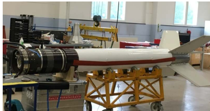
Figure 7. FOS instrumentation of the motor case of Improved Orion second stage.
