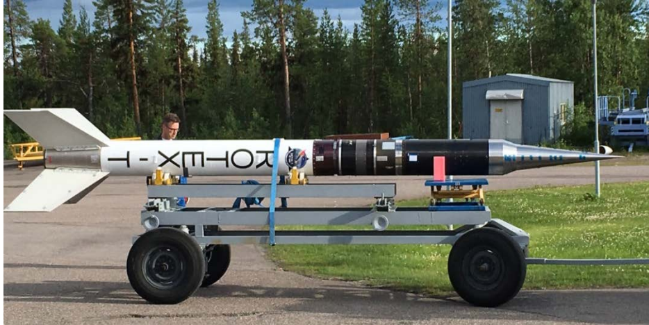
Figure 2. ROTEX-T payload mounted to second stage.
