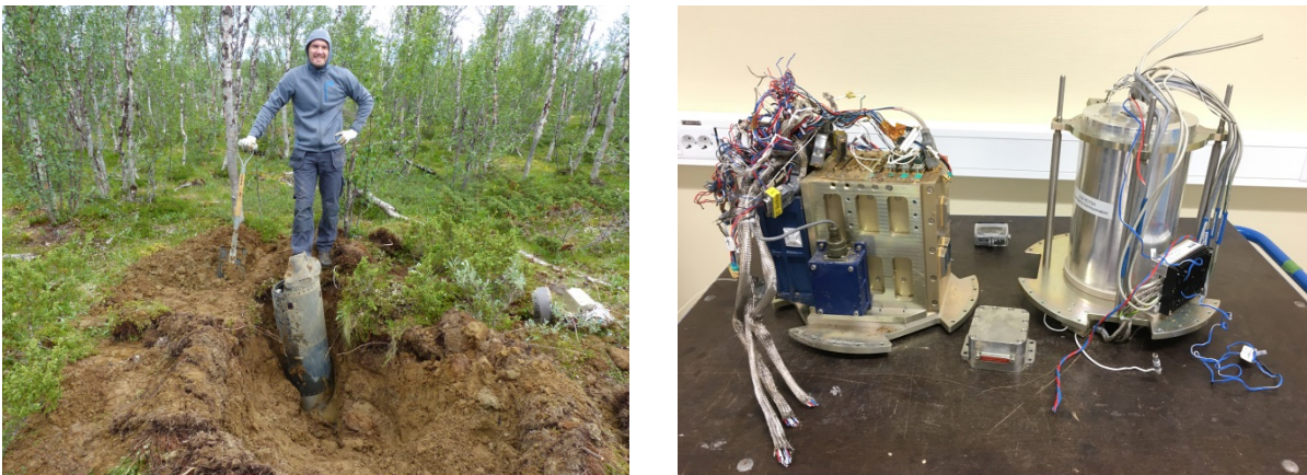
Figure 27. ROTEX-T payload and data acquisition systems after landing without parachute.
