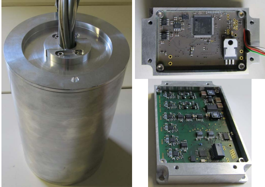
Figure 17. High-speed data acquisition system main unit (left) and front-end electronic boxes (right).
