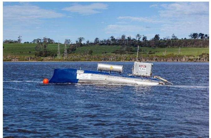
Fig. 13 The operational MAKO Turbines test barge attached to the low flow mooring
