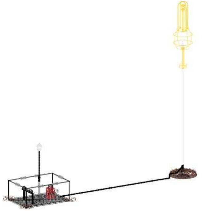
Fig. 3 The steel frame housing the ADCP attached to L-shaped mooring (not to scale)
