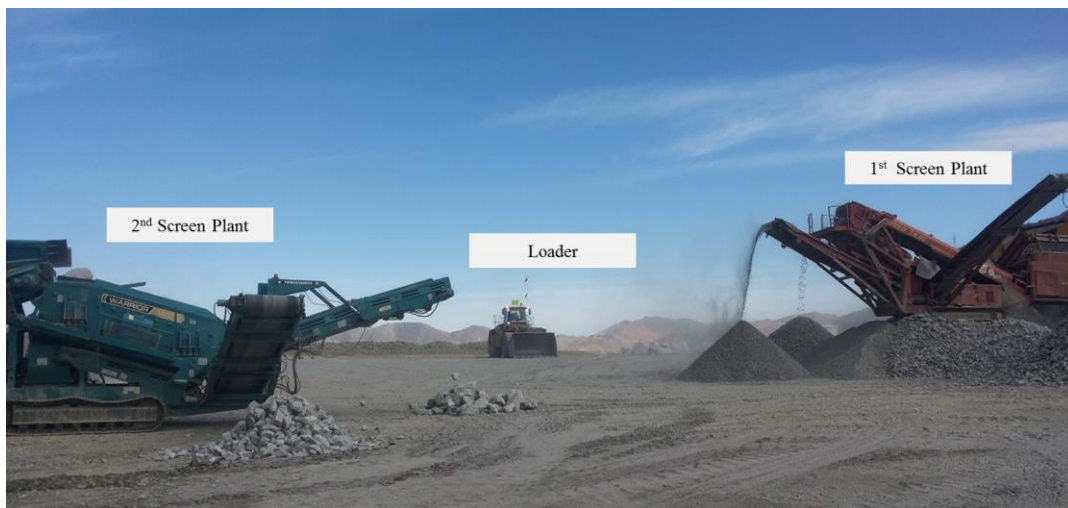
Figure 5-5. Equipment used for validation of preferential grade by size responses at industrial scale (Appendix B).
