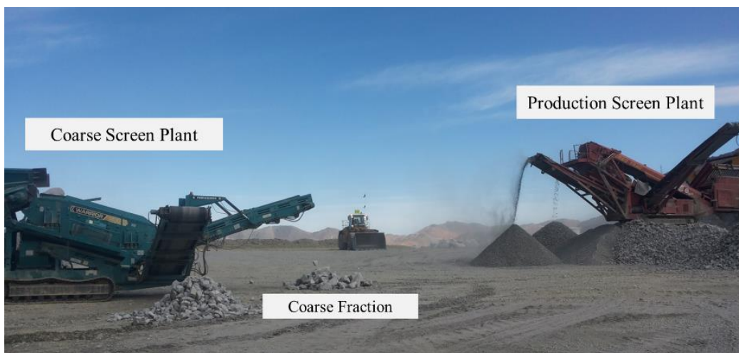
Figure B-1. Second screening unit (green) to address low production screen efficiencies (red).
