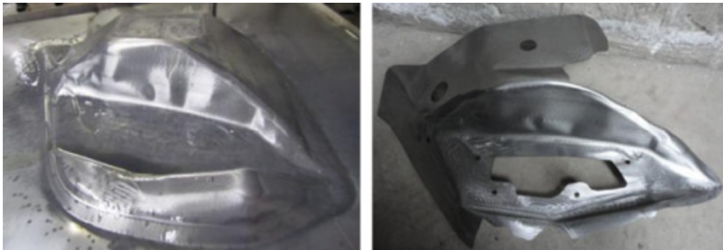
Figure 2-19 The processed taillight bracket: (a) fabricated part via ISF (b) laser trimmed part [67].
