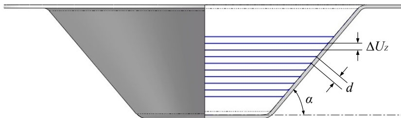
Figure 4-2 Diagram of tool marks on the inner part face.
