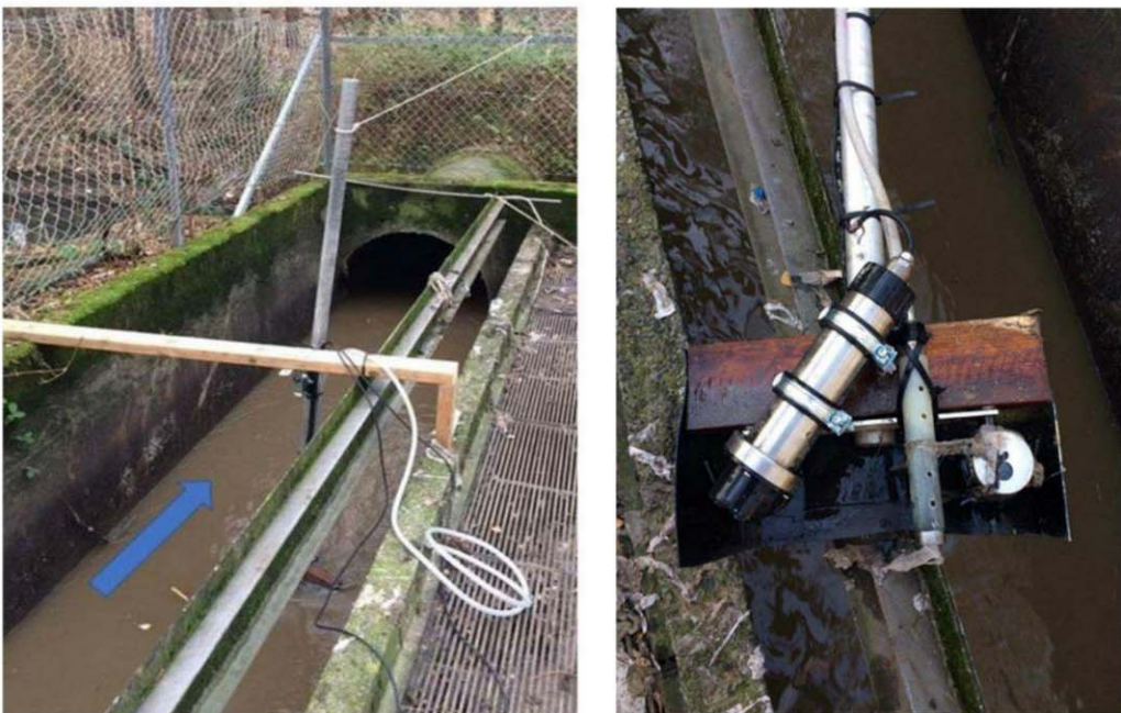
Fig. 1. Left: In-situ sensor installation (blue arrow indicates the flow direction). Left: configuration of the AN-NISE and Solitax Hach sensors (right).
