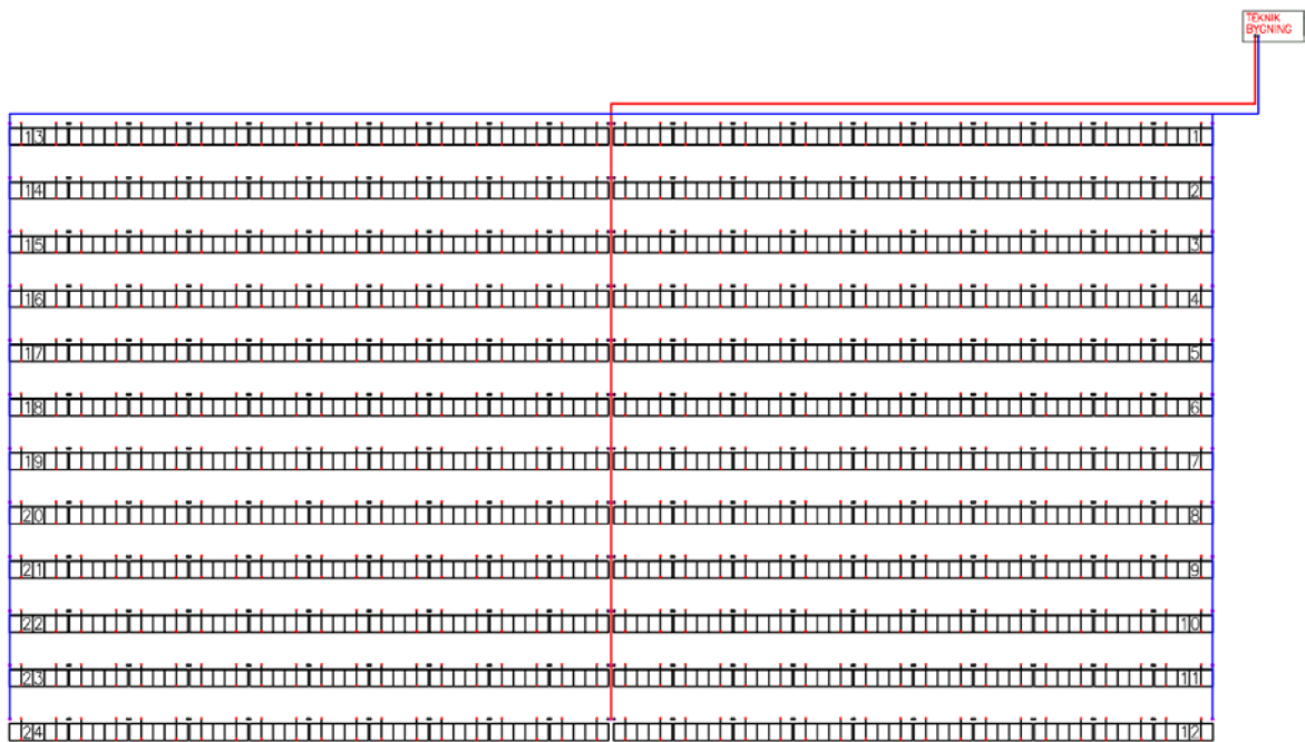
Figure 2: Layout of Høje Taastrup solar collector field: blue and red lines represent supply and return pipes respectively (adapted from Arcon-Sunmark A/S).
