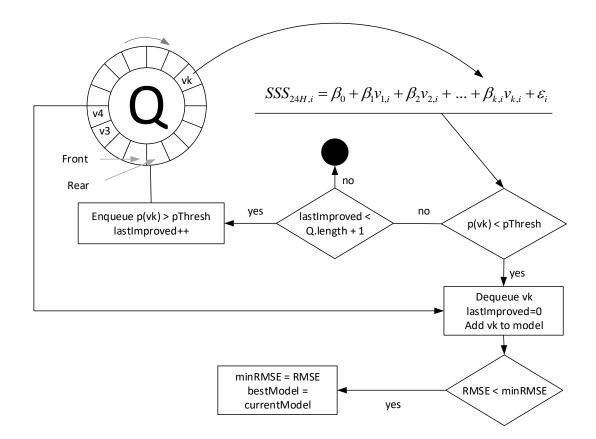
Figure 29: Generation of outcome prediction model by adding or removing predictors iteratively and testing them in a qMLR model. It terminates when remaining possible combinations with the current model no longer improve RMSE.
