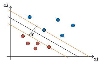
Figure 36: Support Vector Machine example in two dimensions, separated by a line which becomes an n-dimensional hyperplane when n parameters are present. The area between orange lines is the margin and data points closest to the margin are the support vectors.
