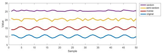
Figure 5: Signal resemblance illustration. Computing the correlation coefficient of the original signal (blue) with itself will result in r = 1. Comparing it to the inverse (red), the correlation is r = -1.
