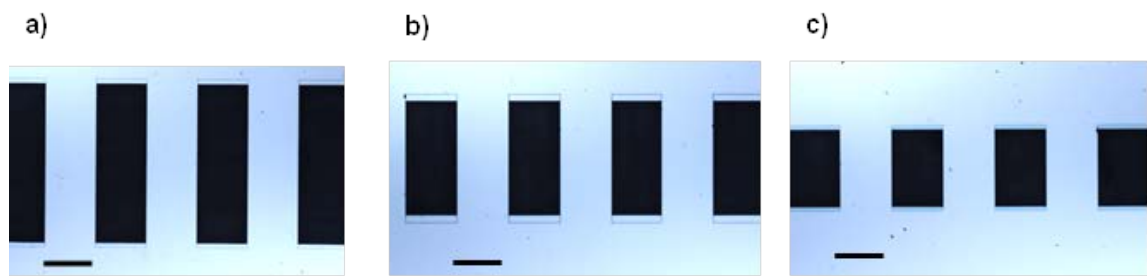
Figure 4.3 Optical microscope images of the microbridge fabricated during this thesis. Scalebar 300 \mu m
