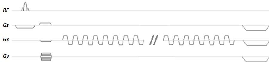
Figure 6.2: Pulse sequence diagram of the EPSI-FID with ETL = 128.
