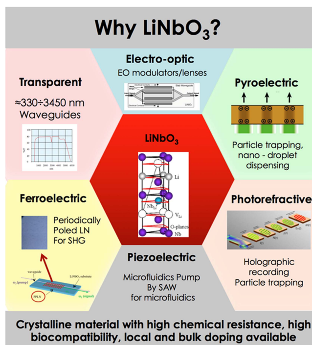
Figure 3. The main properties of lithium niobate (LiNbO 3 ).
