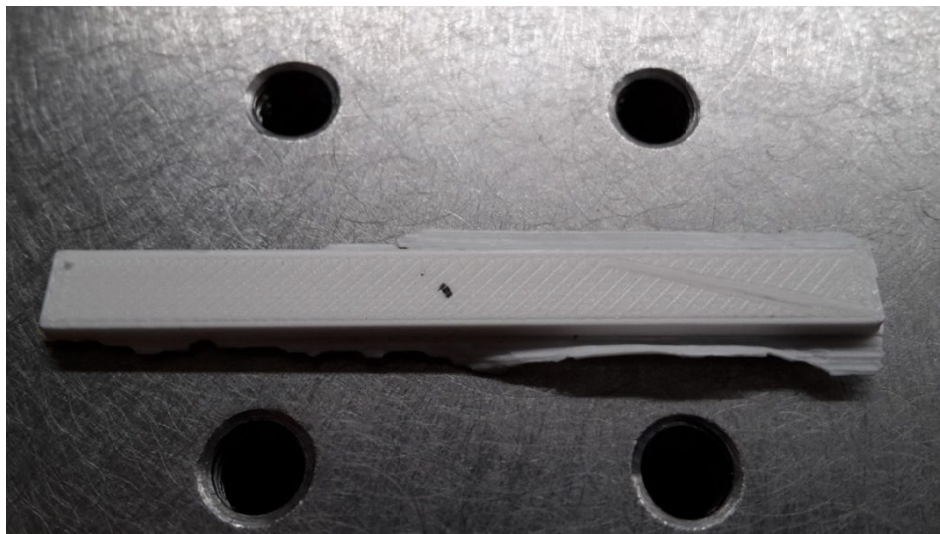
Figure 4: 3D printed PLA block for inspection. Dimensions are designed as 5 mm \times 50 mm \times 2 mm (W \times L \times H). It has been marked with a black dot in the center for recognition.
