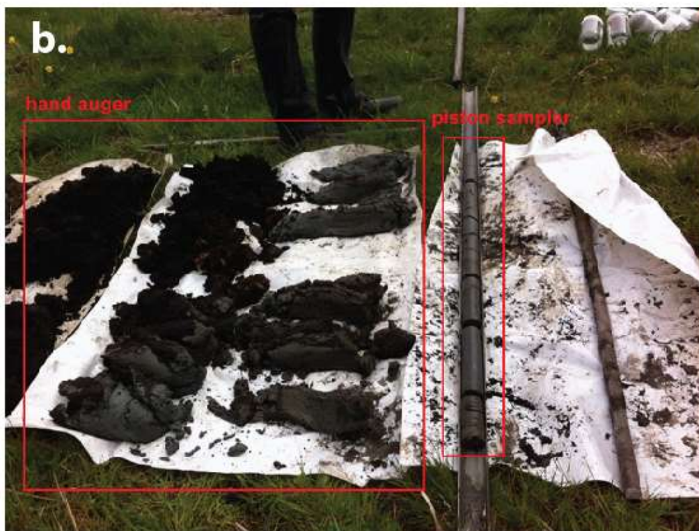
Figure 5. Origin of the core samples. a. Overview of the sample locations on the Walcheren peninsula in the Netherlands. b. Collected sediment at location B08, retrieved using a hand auger (on the left, for sediment above the water table) and piston sampler (on the right, for below the water table).
