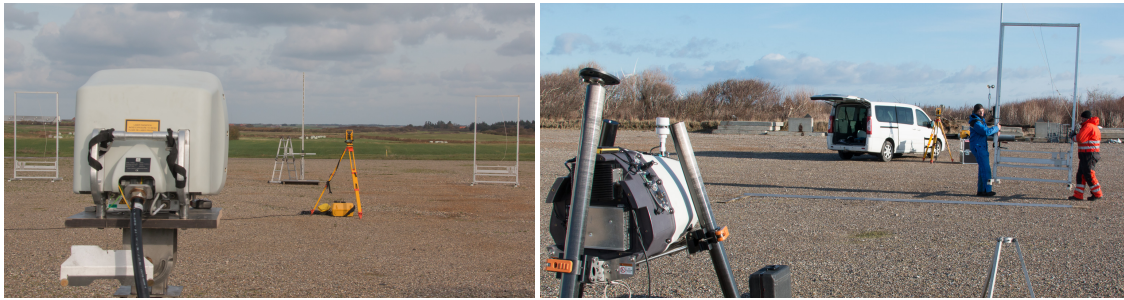
Figure 4. Field testing of the 5B (left) and ZDM (right): inclinometers calibration and beam trajectory verification.
