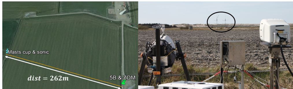
Figure 5. Calibration measurement setup at DTU Wind Energy's test site, Høvsøre, Denmark. Left: Google Earth image; Right: the ZDM and 5B lidars.
