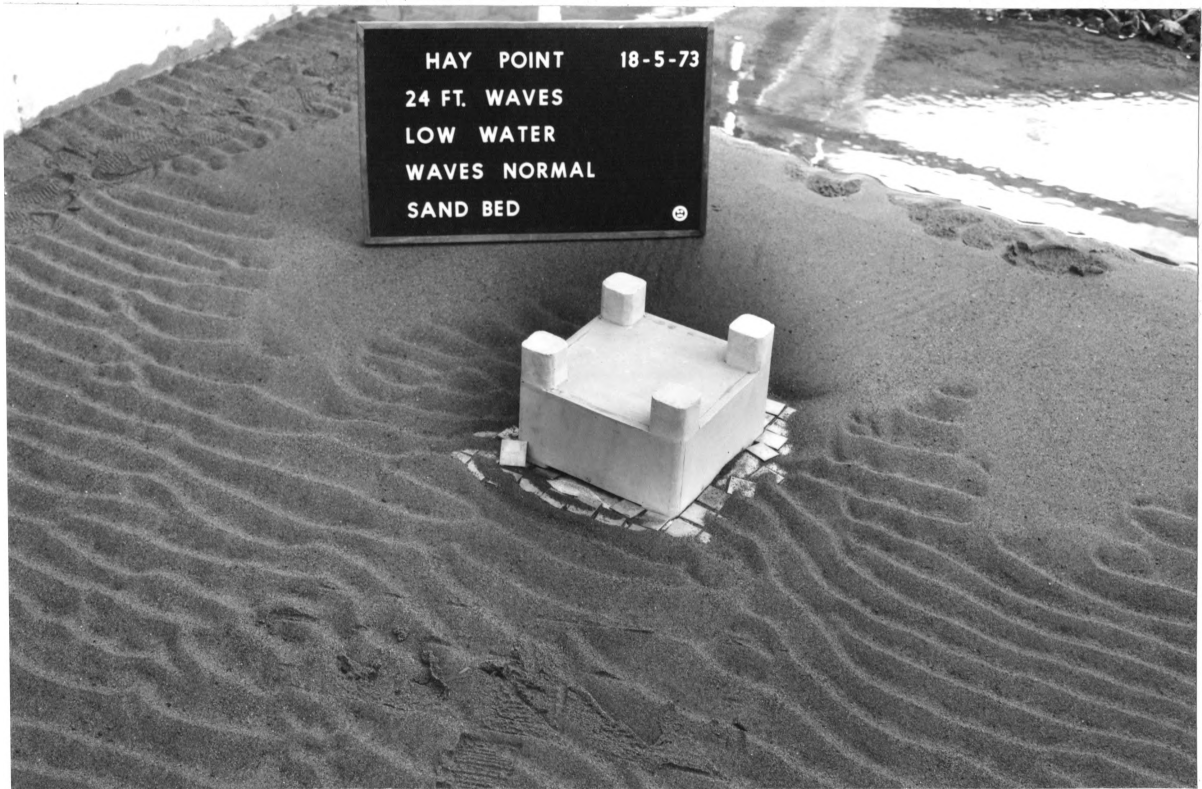
PLATE 21. SCOUR TESTS ON APPROACH CAISSON; SEA-BED OF COARSE SAND; LOWERED FOUNDATION AND BOTTOM GAPS OPEN. FRONT VIEW AFTER ONE HOUR'S TESTING AT LOW WATER WITH 24 FT WAVES APPROACHING IN DIRECTION NORMAL TO BERTHLINE.
