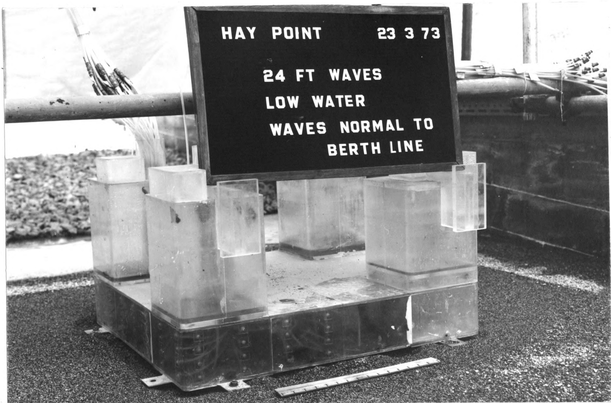
PLATE 3. SCOUR TESTS ON BERTH CAISSON WITHOUT PROTECTION. FRONT VIEW AFTER ONE HOUR'S TESTING AT LOW WATER WITH 24 ft WAVES APPROACHING IN DIRECTION NORMAL TO BERTHLINE.
