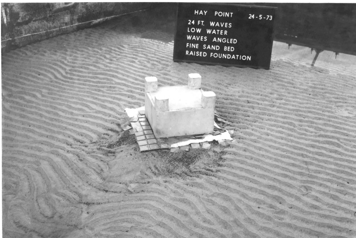
PLATE 26. SCOUR TESTS ON APPROACH CAISSON; SEA-BED OF FINE SAND; RAISED FOUNDATION AND BOTTOM GAPS CLOSED. REAR VIEW AFTER ONE HOUR'S TESTING AT LOW WATER WITH 24 FT WAVES APPROACHING AT 45^{\circ} ANGLE.
