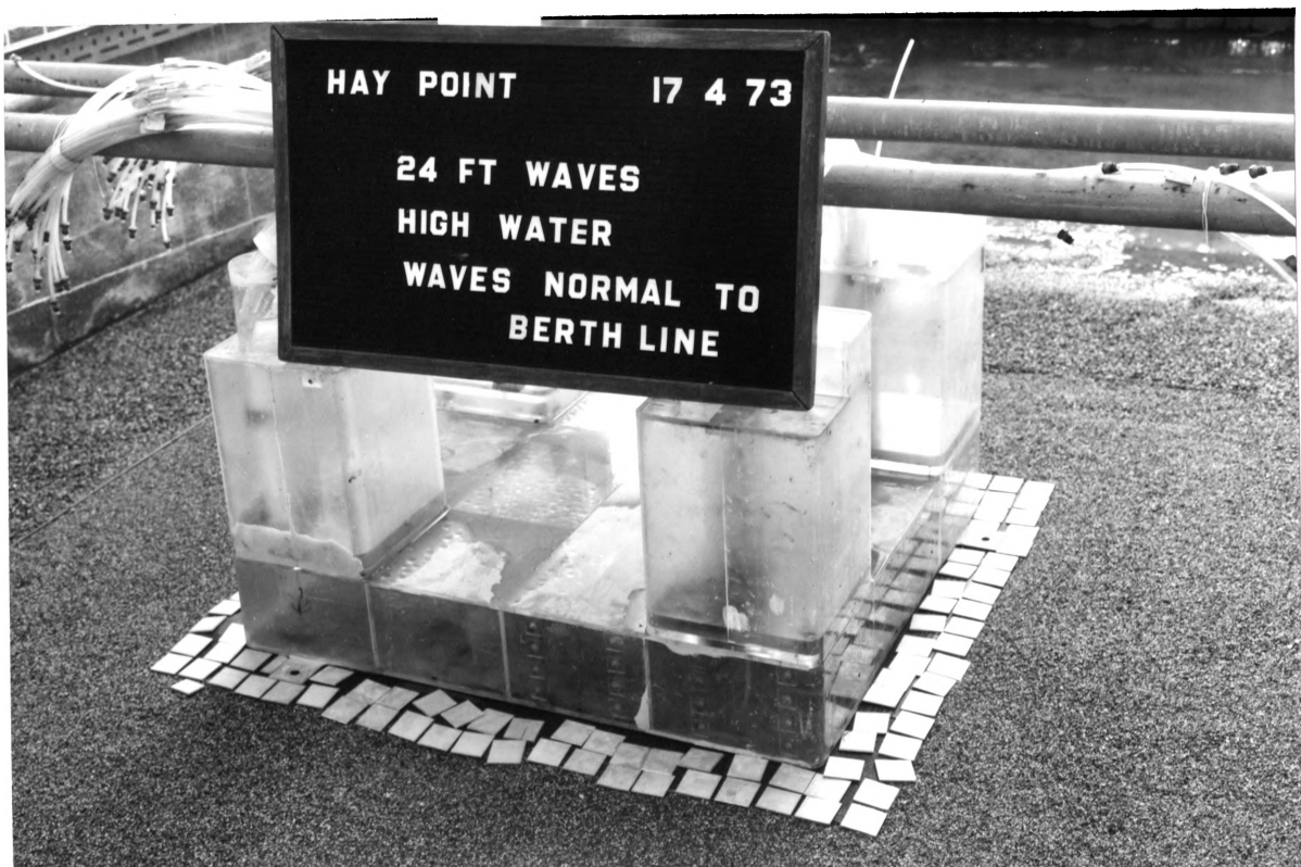
PLATE 14. SCOUR TEST ON BERTH CAISSON WITH SCOUR PROTECTION INSTALLED. REAR VIEW AFTER ONE HOUR'S TESTING AT HIGH WATER WITH 24 FT WAVES APPROACHING IN DIRECTION NORMAL TO BERTHLINE.
