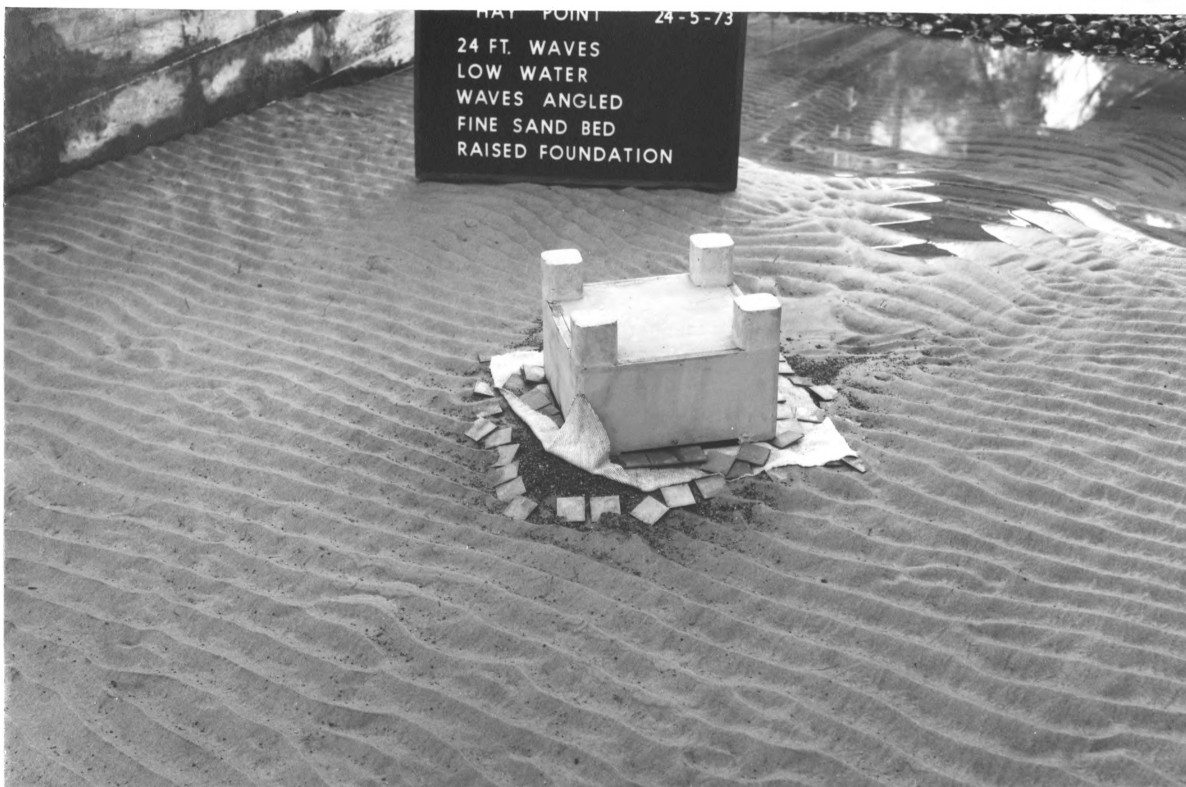
PLATE 25. SCOUR TESTS ON APPROACH CAISSON; SEA-BED OF FINE SAND; RAISED FOUNDATION AND BOTTOM GAPS CLOSED. FRONT VIEW AFTER ONE HOUR'S TESTING AT LOW WATER WITH 24 FT WAVES APPROACHING AT 45^{\circ} ANGLE.
