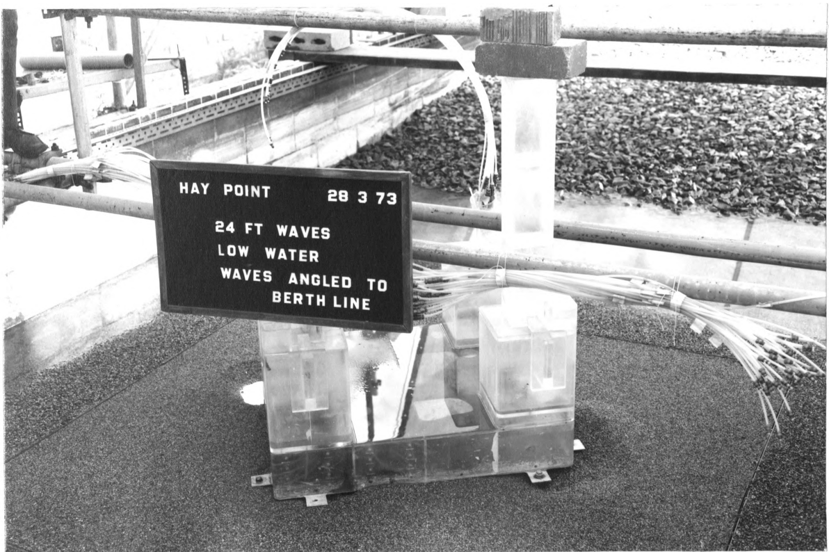
PLATE 5. SCOUR TESTS ON BERTH CAISSON WITHOUT PROTECTION. FRONT VIEW AFTER ONE HOUR'S TESTING AT LOW WATER WITH 24 FT WAVES APPROACHING FROM E.S.E.
