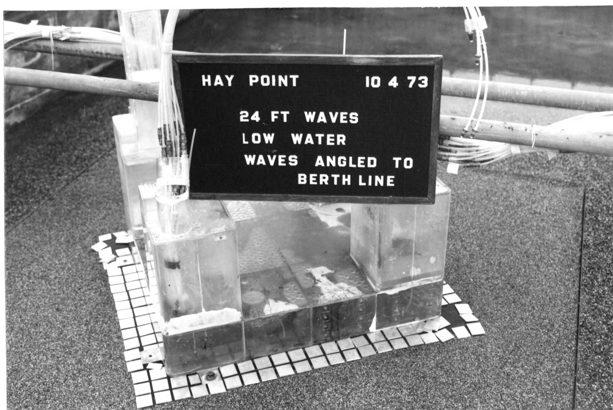
PLATE 12. SCOUR TEST ON BERTH CAISSON WITH SCOUR PROTECTION INSTALLED. REAR VIEW AFTER ONE HOUR'S TESTING AT LOW WATER WITH 24 FT WAVES APPROACHING FROM E.S.E.
