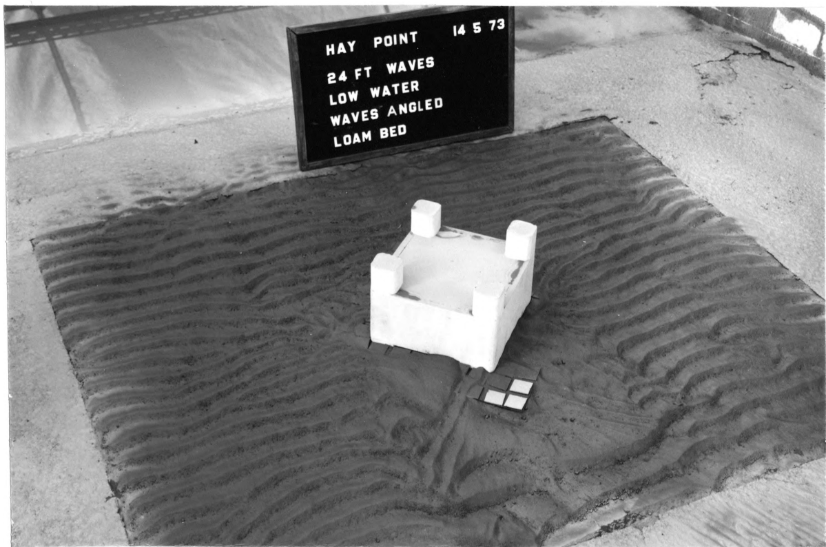
PLATE 20. SCOUR TESTS ON APPROACH CAISSON; SEA-BED OF LOAM; LOWERED FOUNDATION AND BOTTOM GAPS OPEN. REAR VIEW AFTER ONE HOUR'S TESTING AT LOW WATER WITH 24 FT WAVES APPROACHING AT 45^{\circ} ANGLE.
