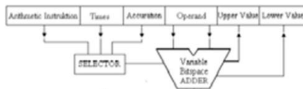
FIGURE 2. Block diagram of computational arithmetic adder variable bitspace
