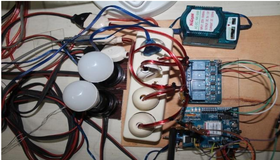
FIGURE 6. The devices of automation system for monitoring and home appliances control via sms
