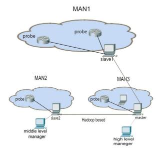
FIGURE 2. The architecture of Hadoop policy based network management
