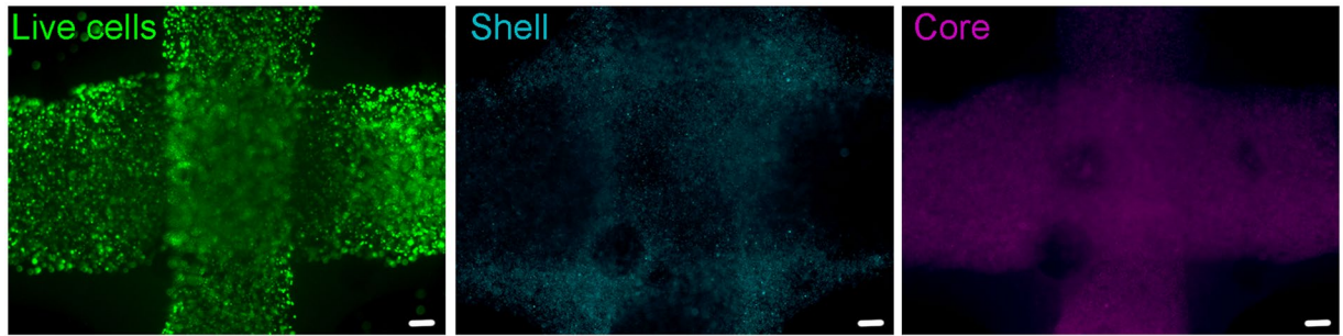
Figure 7. Core/Shell printing facilitates a layer by layer deposition of cell-laden hydrogels with structural integrity. Representative epifluorescent image of Calcein-AM (green channel) stained cells after 7 days from printing. The Shell and the Core has been differently labeled with fluorescent beads (cyan channel for Shell, violet channel for Core) to estimate the compartmentalization. An epifluorescent Olympus IX70 inverted microscope with a SPOT Diagnostic RT-Slider camera and SPOT Diagnostic software was used with an Olympus 4X UPlanFL NA0.13 objective lens.
