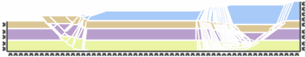
Figure 5.8: Deformed James Bay dykes
