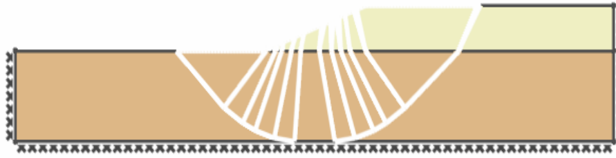
Figure 4.7: Failure Mechanism in Slope
