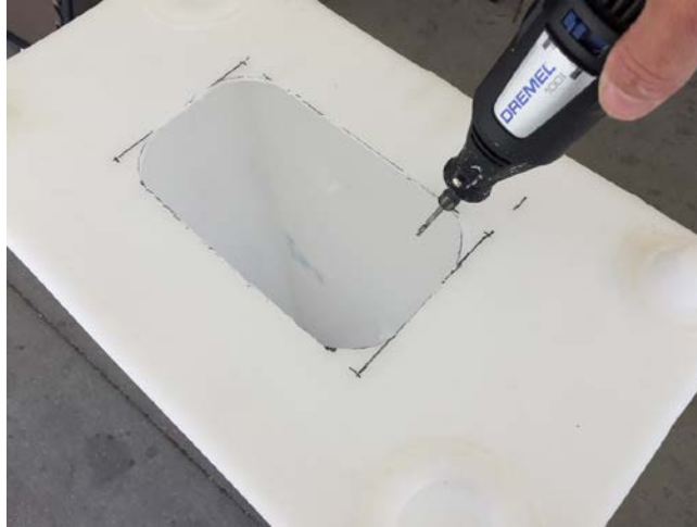
Figure 19: Cutting the Access Hole
