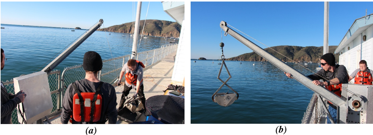
Figure 2.6 (a) The grab was attached to the steel cable on the crane arm. (b) The arm was slowly rotated over the pier. The winch mechanism can be seen in the lower right-hand corner.
