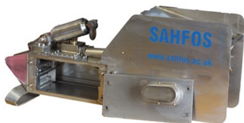
Figure 2.12 The current model of the Continuous Plankton Recorder (CPR). The opening allows for a collection cassette to be easily inserted and removed. [8]
