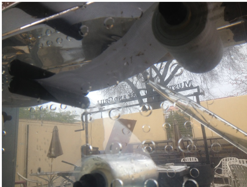
Figure 7.3 Using the turkey baster to release analogues towards the top belt. The baster had a relatively narrow dispersal area, useful for squirting bloodworms.
