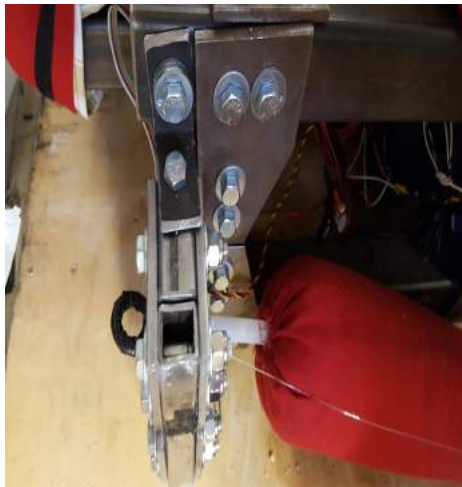
Figure 14.5. Shoulder after Impact
