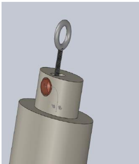
Figure 7.8. Shoulder with pipe connector and eye bolt (Original design, current uses a 90° shaft clamp instead of the pipe connection)
