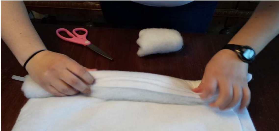
Figure 13.2. Rolling the batting around polyethylene tubing.
