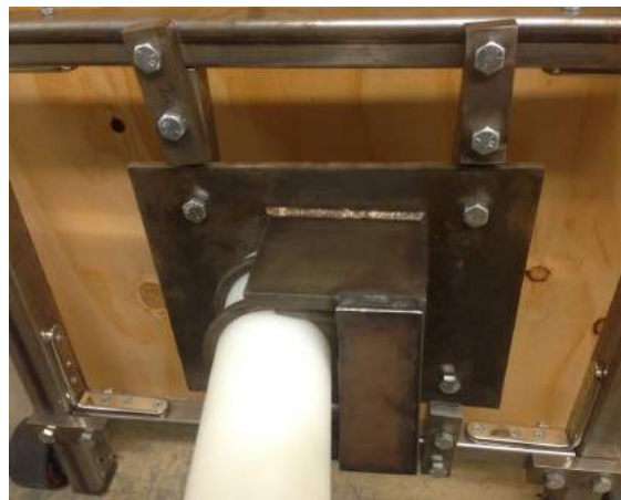
Figure 7.9 Pole Holder in Containment, with the pole attached.
