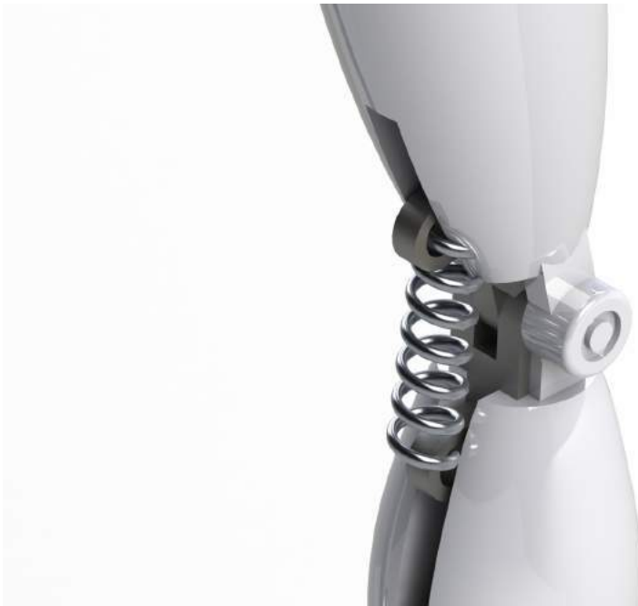
Figure 4.2.7. Compression spring and rotary damper at the knee
