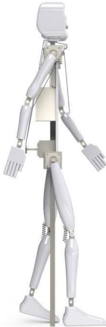
Figure 4.2.6. Side view of the mannequin showing mechanical tendon assembly.
