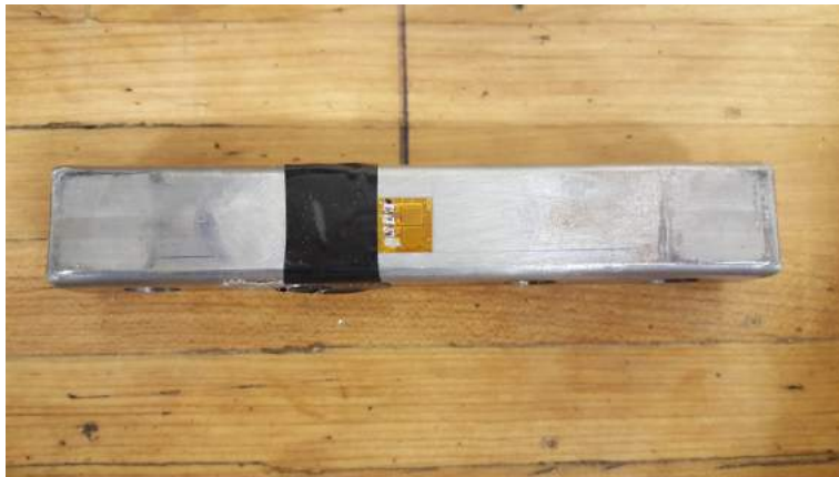
Figure 14.1. Foil strain gauge applied to the right shoulder of the test target.
