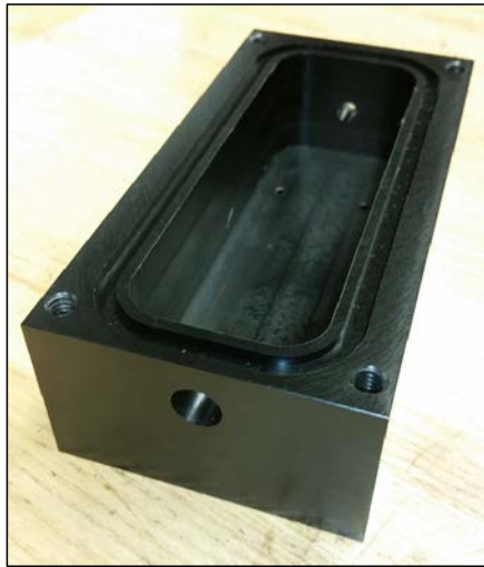
Figure 61. Second Revision of Motor Housing CNC Machined from Delrin.
