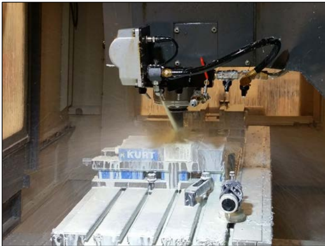
Figure 59. First Motor Housing Revision being CNC Machined on the Haas.
