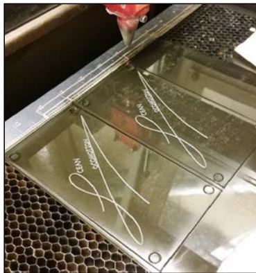
Figure 60. Laser Cutting Motor Housing Top.
