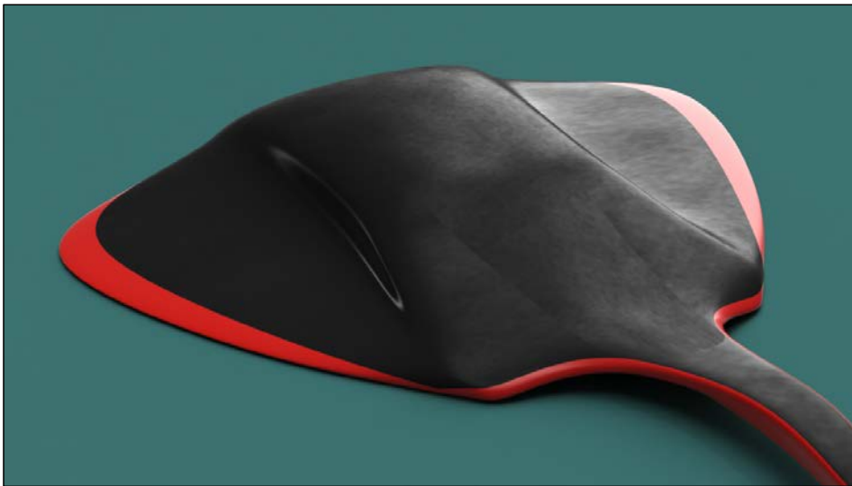
Figure 33. ROV Concept Showing Electroactivated Polymer Location for Simulated Fin Motion.
