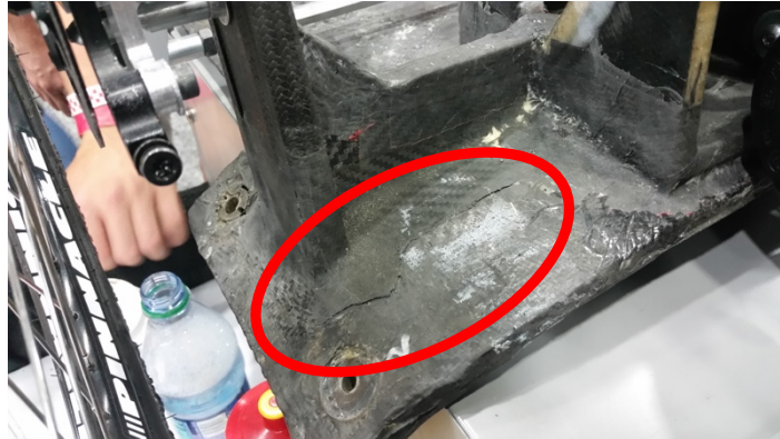
Figure 11. Photo of the steering plate taken during competition after the car was brought in for repairs. A structural failure can be seen in the carbon fiber steering system.
