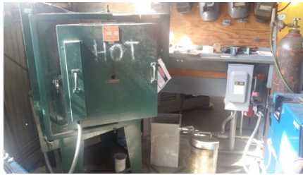
Figure 45. The hangar furnace. It is capable of reaching temperatures up to 2000°F which makes it perfect for heat treating.
