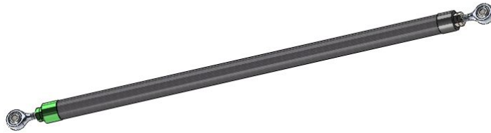
Figure 39. The tie rod assembly that connects the two wheels. The short tie rod connects the steer to one of the wheels to initiate turning.
