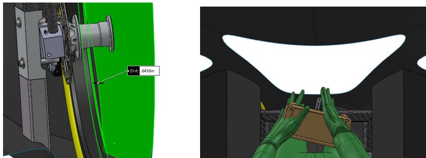
Figure 54. Size testing performed in CAD. Both passed the specification with the minimum distance to the chassis being 0.64 inch and no interference with visibility.
