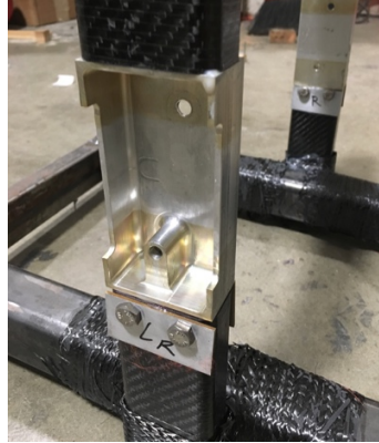
Figure 55. Modifications made to the subframe to increase its reliability and strength.
