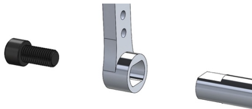
Figure 37. A close up of the mating surfaces of the steering column to the steerer.
