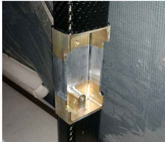
Figure 43. Aluminum Uprights with Alodine 1201 created chrome conversion surface
