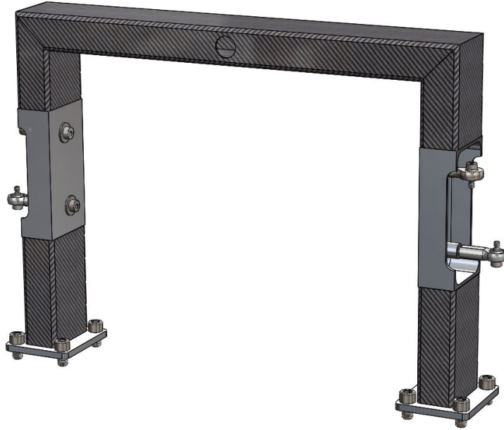
Figure 26. A rendering of the subframe assembly. It is characterized by the carbon tubes, uprights, rod ends, lugs, and base flange.
