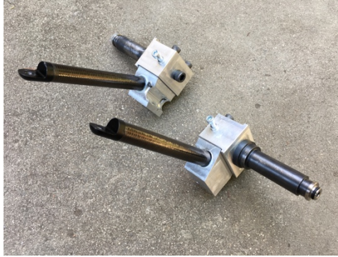
Figure 49. Left and right Axle Assemblies completely manufactured.
