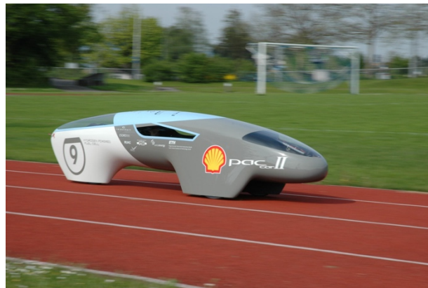
Figure 14. PAC-Car II being tested on a track by the ETH Zurich Supermileage team.
