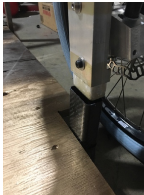
Figure 53. The uprights pulled out of the bottom support due to poor surface prep and an inadequate bond line thickness.
