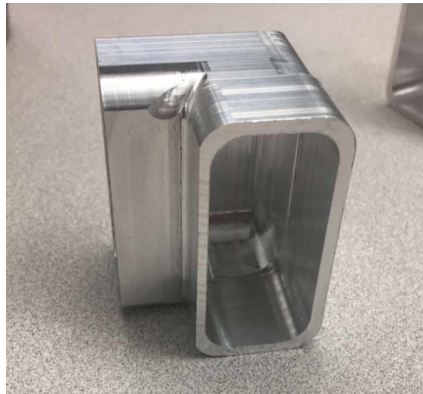
Figure 42. The completed corner lug shortly after finishing its last operation.
