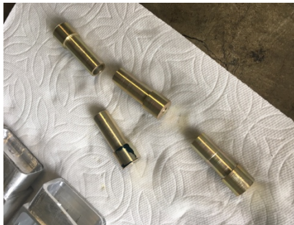
Figure 50. Aluminum tie rod bungs treated with AlumiPrep and Alodine to produce a better bonding surface.
