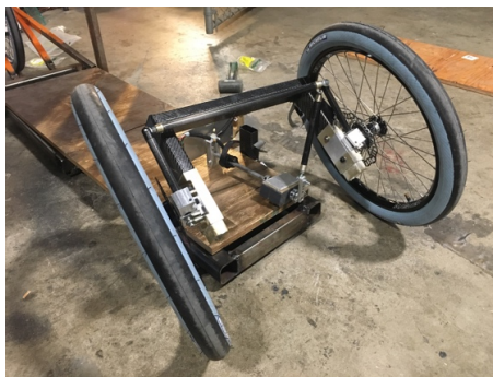
Figure 52. The broken steering system after drop test. The uprights pulled out of the bottom tubes.
