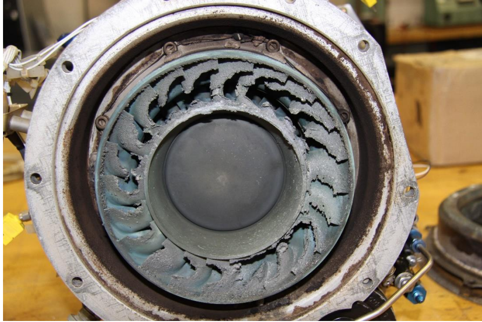
Figure 6. Stator for the power turbine, almost completely disintegrated
