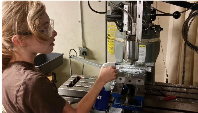
Figure 60. Base plate machining setup
