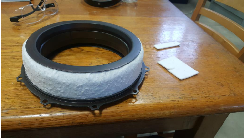
Figure 65. Thermal insulation wrapped around containment ring prior to installation
