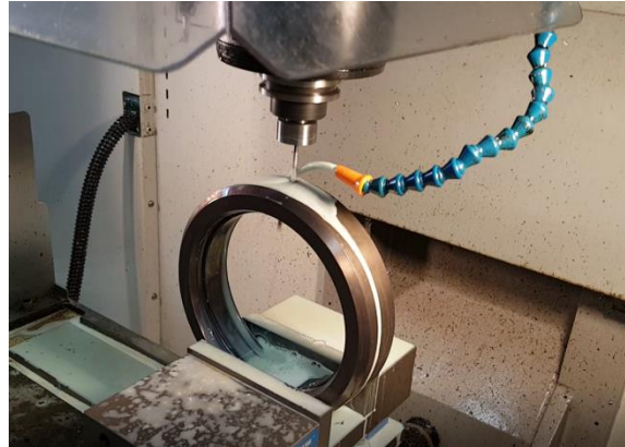
Figure 57. Final Machining of Actual Containment Ring
