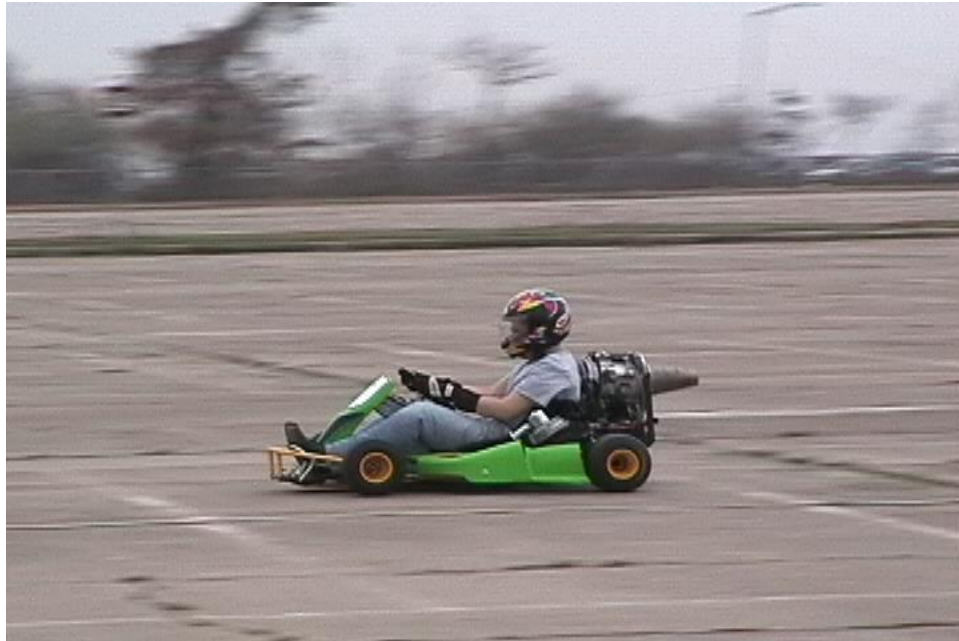
Figure 9. The original Turbokart, powered by a JFS-100 engine [9]
