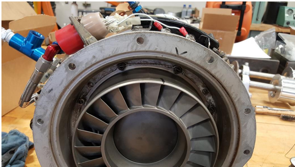
Figure 64. IGV ring installed in the gas-generator assembly, with the bolts safety-wired
