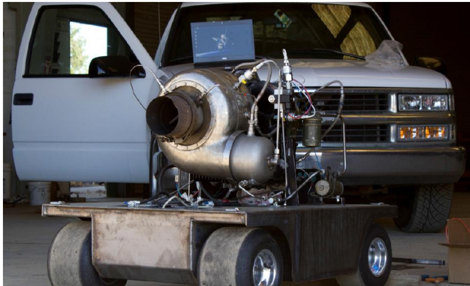
Figure 11. GTP350-51 turbine engine upon completion of the 2012 senior project work[11]
