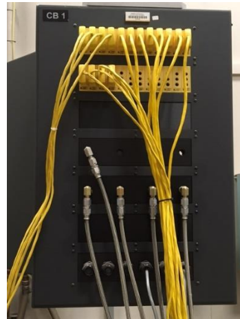
Figure 45. Inputs to dyno control box
