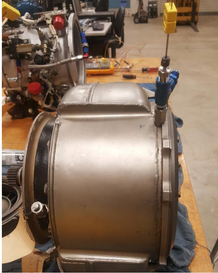
Figure 67. Stage 4 instrumentation installed in power turbine
