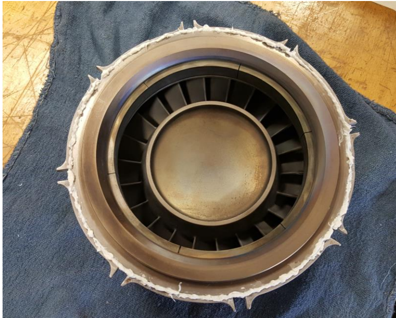
Figure 63. Power turbine IGV ring ready for installation
