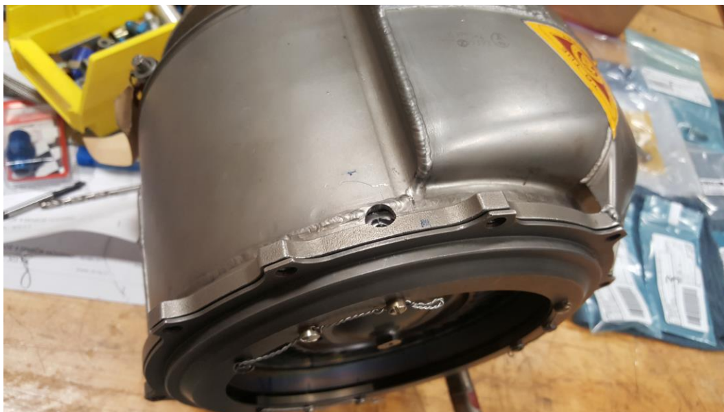
Figure 66. Containment ring installed in power turbine housing
