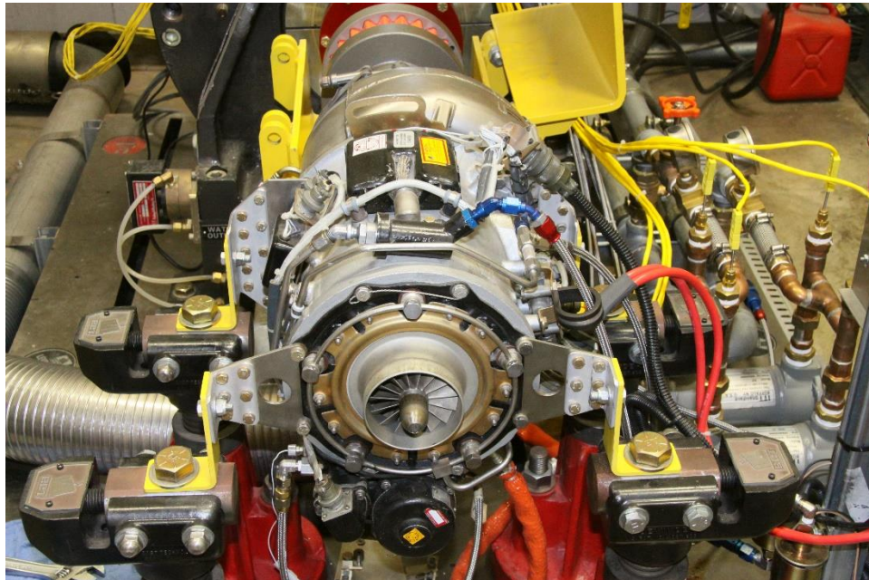
Figure 3. Close-up of the compressor intake after the JFS was installed in Cal Poly's Engines Lab
