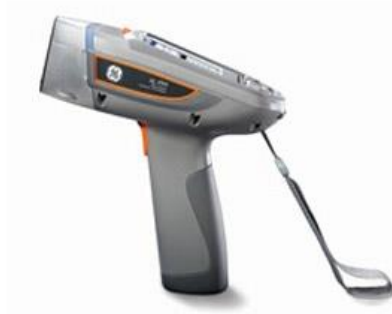
Figure 22. Portable XRF Analyzer [17]
