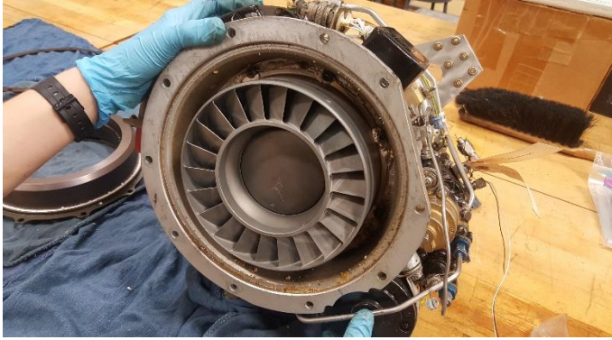
Figure 20. P.T. Inlet Guide Vanes
