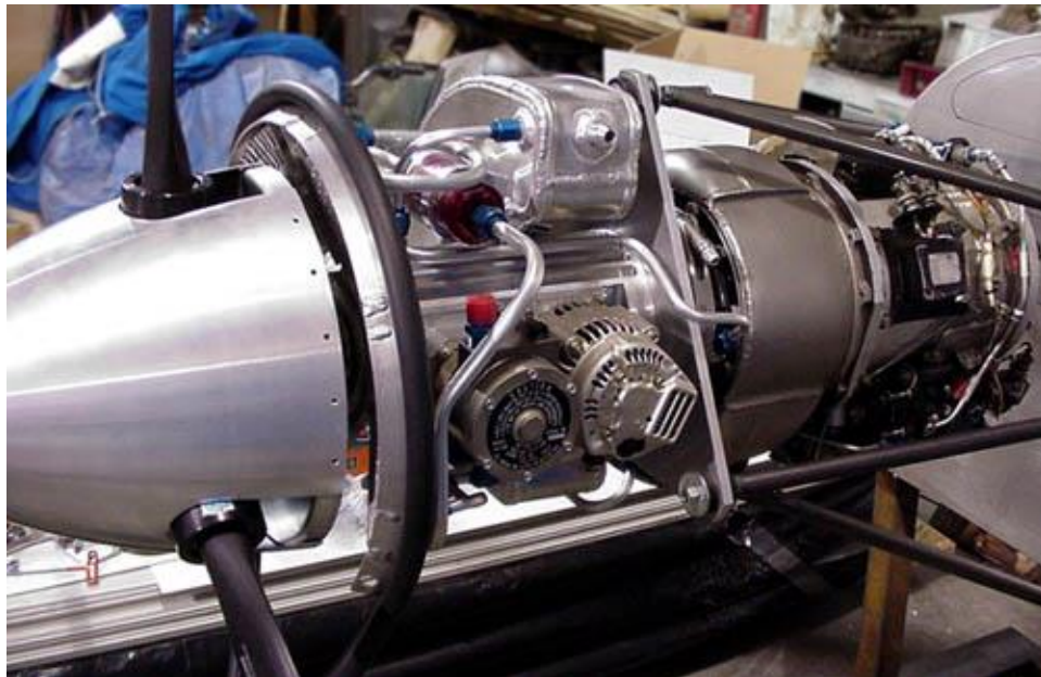
Figure 10. JFS-100 engine driving the propeller of a home-built aircraft [10]
