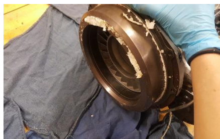
Figure 18. Containment Ring Front
