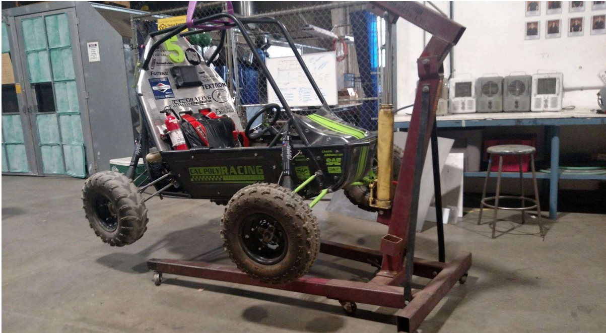
Figure 5. Lifting the Baja car by the roll hoop to allow the team to work at waist height on critical components of the car. Note the lack of significant clearance between the tow hitch and the hydraulic cylinder. We've removed the cylinder in our design, but replaced it with a geometrically identical support beam, which will lock onto the tow hitch of the car and hold it in place.
