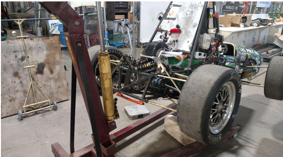
Figure 6. Lifting the Formula E-car with the hoist. It was particularly well balanced, though settled just off level. There were no significant problems lifting this car with the hoist.
