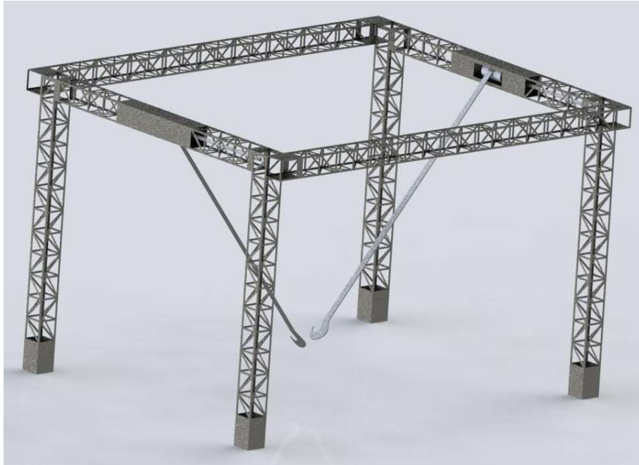
Figure 4. Render of our preliminary design including a four-post lift and two lifting straps.
