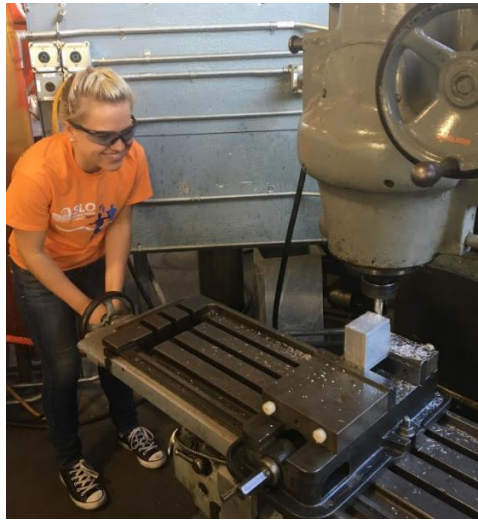
Figure 55: Team member KC Balfour milling stock aluminum to create the frame-to-shaft attachment piece for the back wheels
