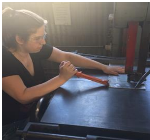
Figure 48: Cutting the sheet metal on a band saw for the back brackets.
