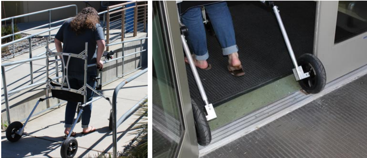
Figure 69: Testing Walker on ADA ramp, Figure 70: Walker through a doorway
