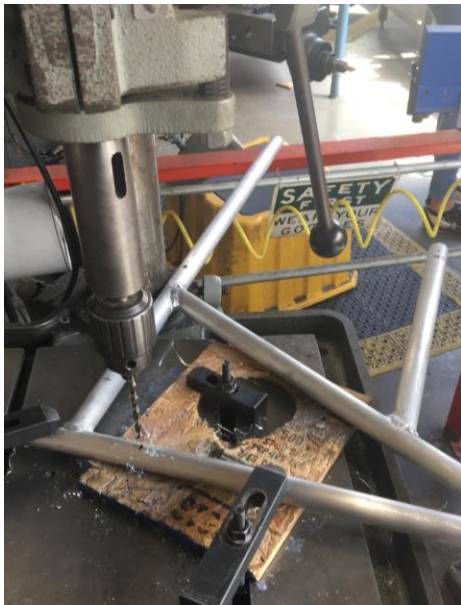
Figures 44 and 45: Frame in drill press for drilling holes.
