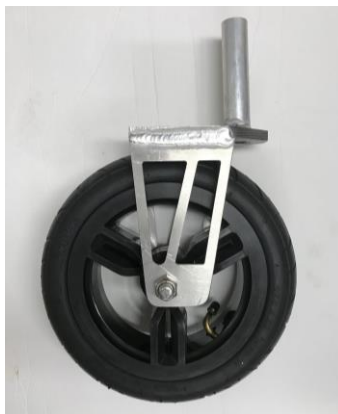
Figure 54: Welded and Assembled Front Caster/Wheel
