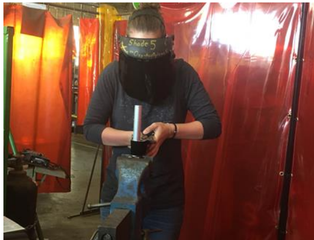
Figure 50: Set-up to bend the back brackets. One inch tubing is held in the vice while the metal sheet is held by two vice grips.
