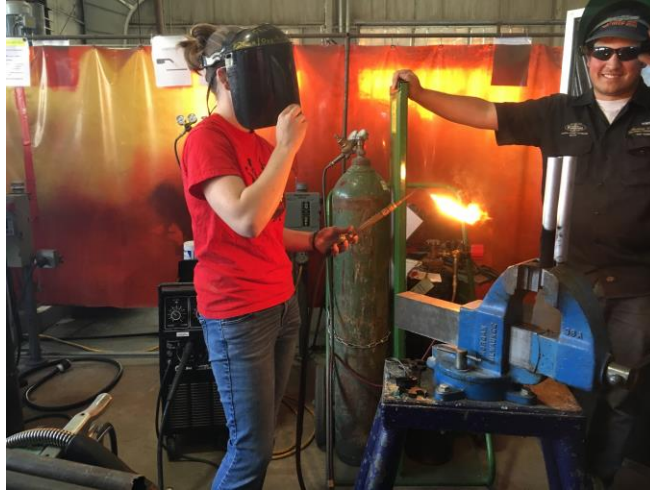
Figure 52: Team member Jayne heating up the front legs, the black layer of ash was used as an indicator that the metal had been annealed.
