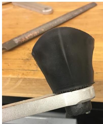
Figure 59: Forearm support from manufacturer, Figure 60: Filed part to fit into the arm connector
