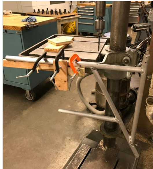
Figures 44 and 45: Frame in drill press for drilling holes.
