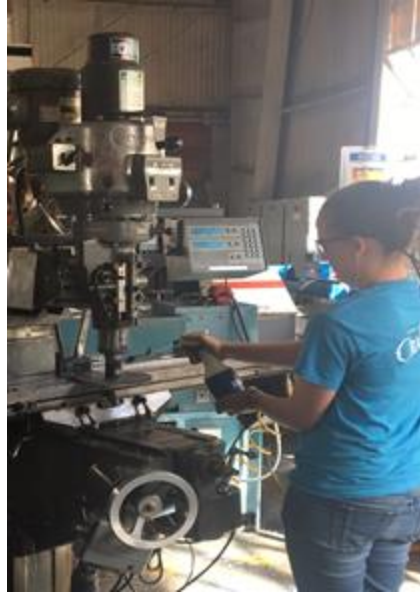
Figure 47: Circular Slotting Saw on a mill used to cut the slot in the center piece where the horizontal bars connect
