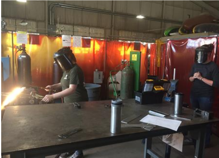
Figure 49: Annealing of the sheet metal using an Acetylene torch.
