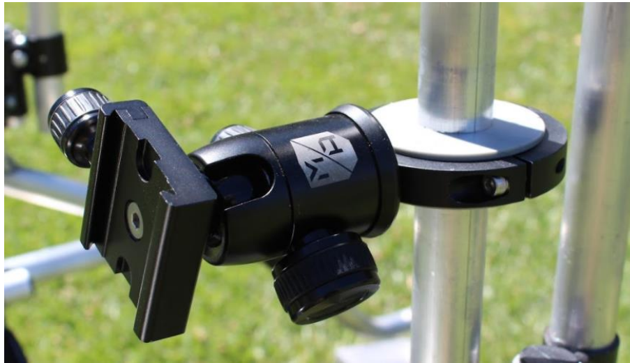
Figure 65: Custom Communication Device Holder/Mount, from left to right Mob Armor tablet mount, rotational piece, and frame attachment.
