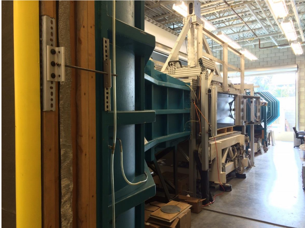
Figure 24. The Cal Poly low speed wind tunnel with the test section doors open. Air flow is from left to right.
