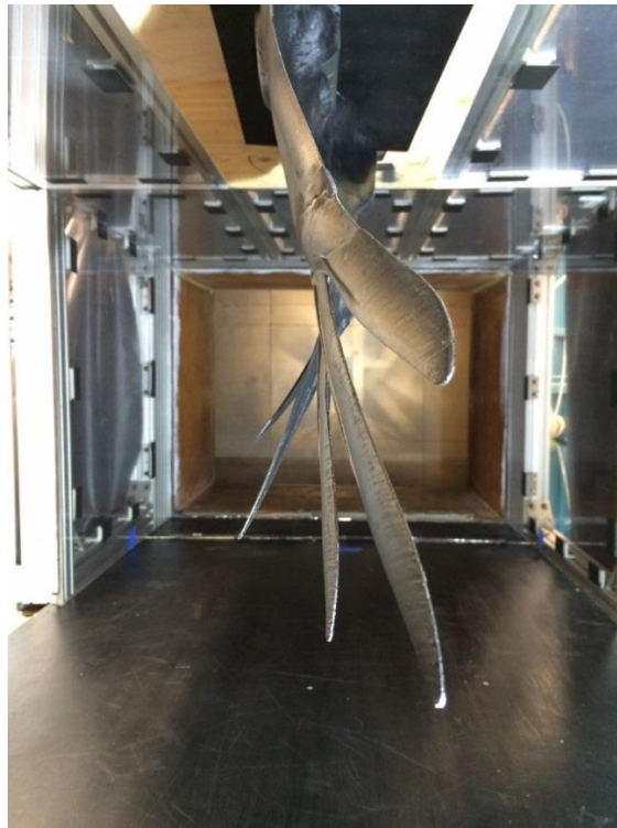
Figure 23. Final aerodynamic test model mounted in the Cal Poly low speed wind tunnel. Rear view.
