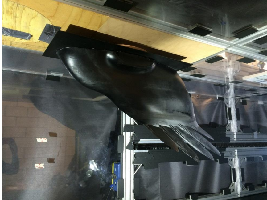
Figure 22. Final aerodynamic test model mounted in the Cal Poly low speed wind tunnel. Side view.
