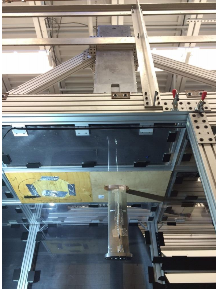
Figure 25. Overview of the linear drive system with mounting plate extended.
