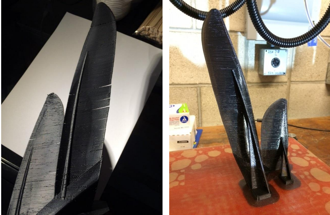
Figure 20. A comparison between identical parts printed in ABS (left) and T-Glase (right).
