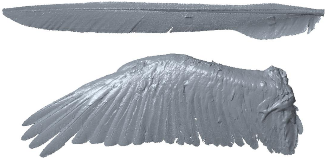
Figure 12. 3D scans of a Brown Pelican wing and primary feather generated by the NextEngine 3D scanner (not to scale).
