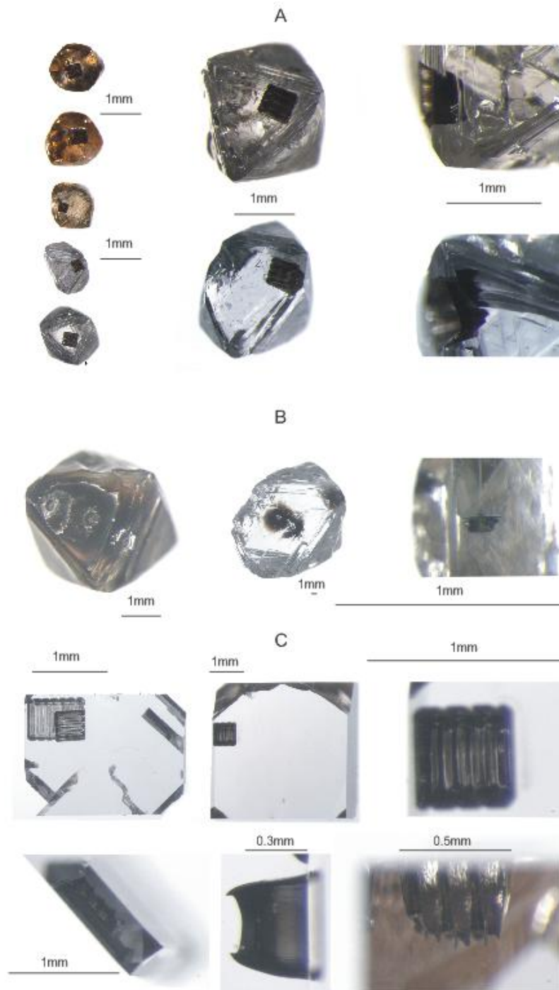
Figure 2.4. Diamonds in this study. A - Diamonds from Canada demonstrating the size of the offline ablation pit. B – Diamonds from Diavik previously analyzed by the GEMOC group using the online laser ablation method. Note the ejecta material remaining behind after ablation. C – Synthetic diamonds analyzed in this study which demonstrate the well proportioned and clean laser pits resulting from the offline ablation technique.
