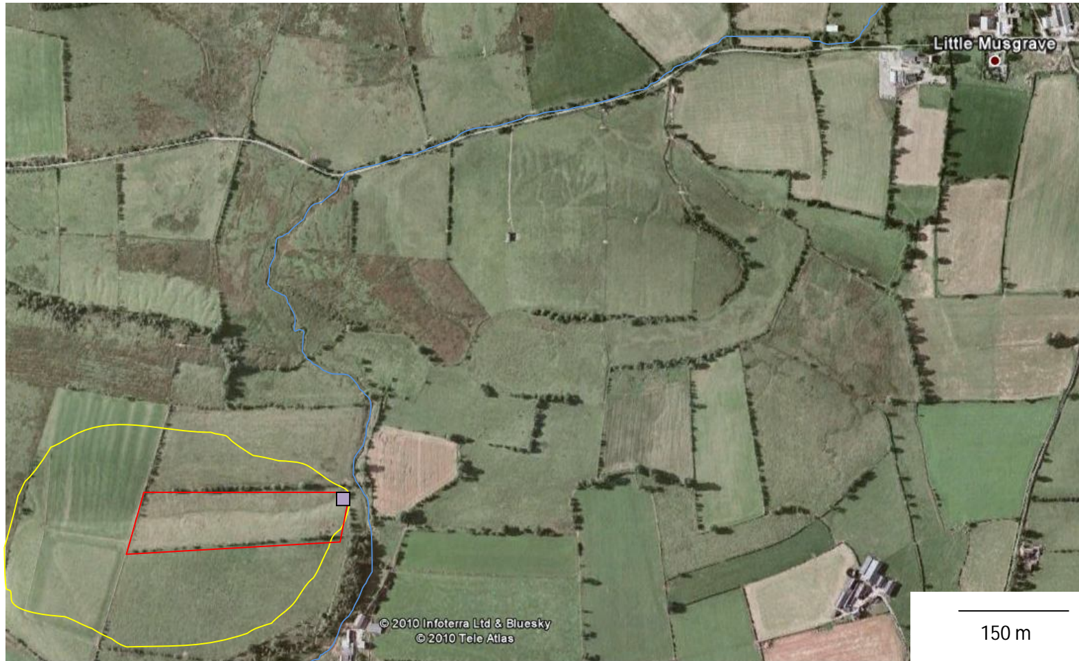
Figure 3.4: Study site at Sykeside Farm (red) in relation to the ephemeral catchment watershed (yellow) and the unnamed stream (blue). Little Musgrave is marked for orientation. The location of the V notch weir and rain gauge is identified by a purple square. (Derived from Google Earth).
