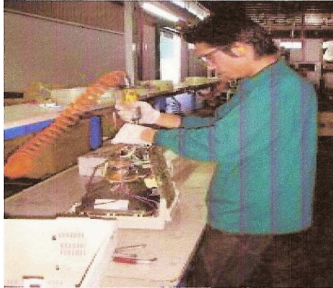
Plate 2.10: Dismantling of used computer at a recycling company in Malaysia. (Source: Reclaimtek (M) Sdn. Bhd.)
