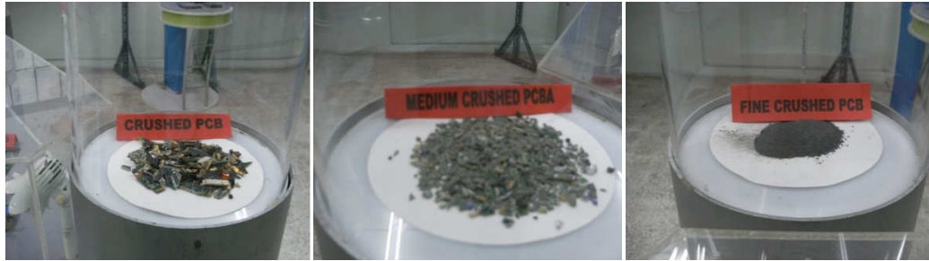
Plate 2.4: Coarsely crushed printed circuit boards. (Source: author - courtesy of Tes-Amm (M) Sdn. Bhd.)
