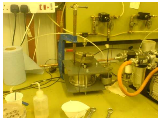
Figure 7.10 – Grout test set up.
