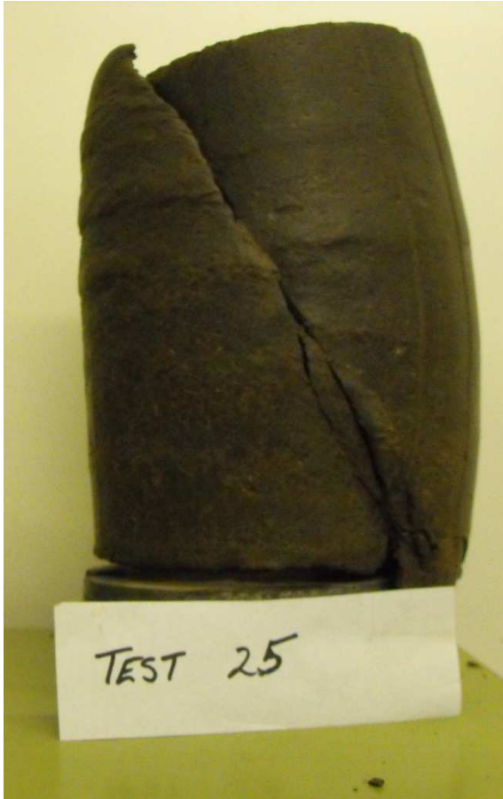
Figure 6.40 – Typical shape of failure on samples tested for with W_{ci} close to 15%.
