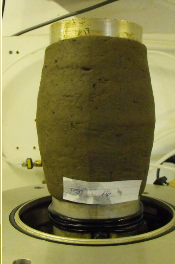
Figure 6.41 – Typical shape of failure on samples tested with W_{ci} close to 20% and 22%.
