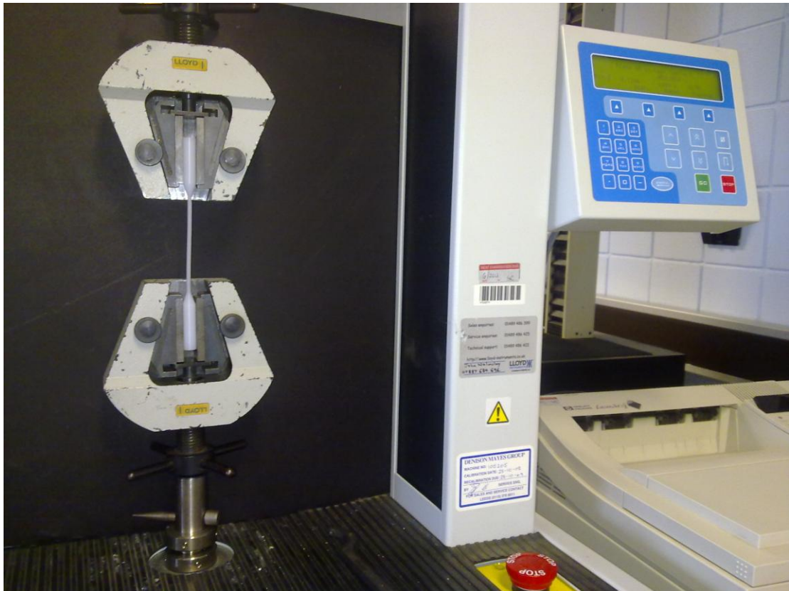
Figure 5.4 Tensile testing machine with a specimen made of UHMWPE mounted
