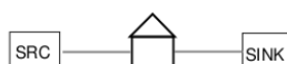
Figure 3.1: In a simple example of EMC the chain of communication would resemble this. [38]
