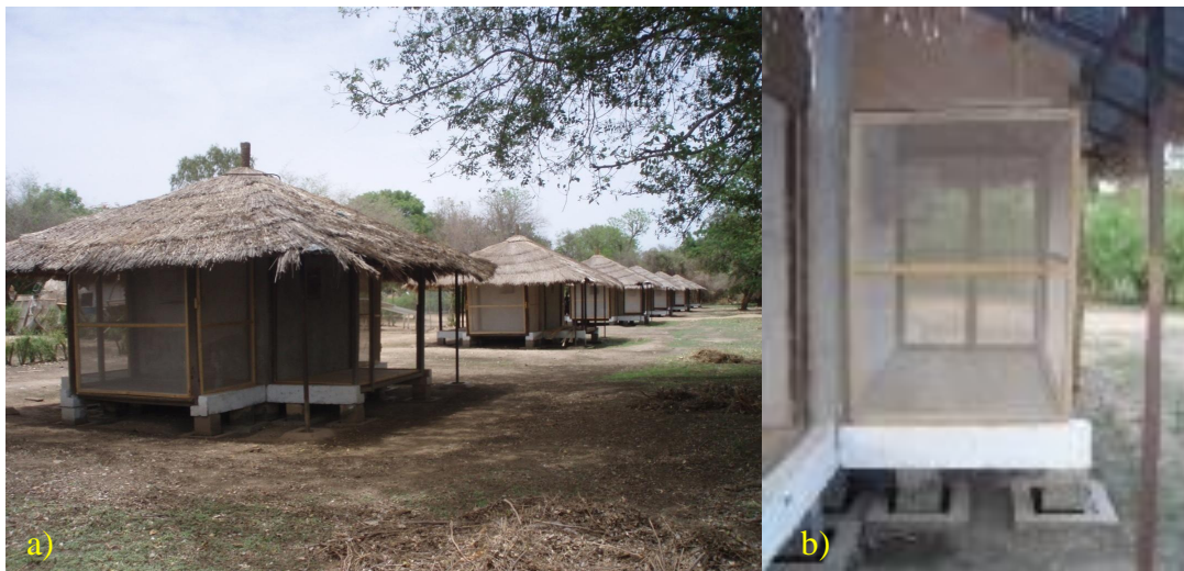
Fig. 3.2 a) Experimental huts at Walikunda, b) Veranda trap with exit trap fixed over window
