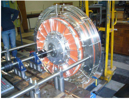
(a) Stator and rotor supporting units
