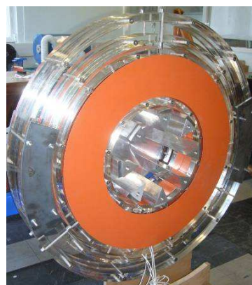
Fig. 7-10. Test rig without front rotor disk.
