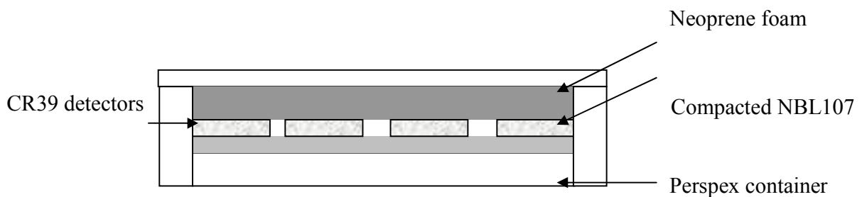
Figure 5.10 Cross sectional representation of apparatus used for CR-39 initial testing
