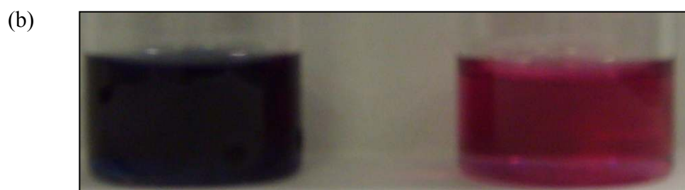
Figure 3.5 – (a) UV/Visible absorbance spectra of 3.1 at t = 0 (red), t = 1 day (green), and t = 7 days (blue) at 5 \times 10^{-4} \text{ mol dm}^{-3} concentration in 10% DMSO in acetone. (b) vials containing the solutions t = 0 (left) and t = 7 days (right).
