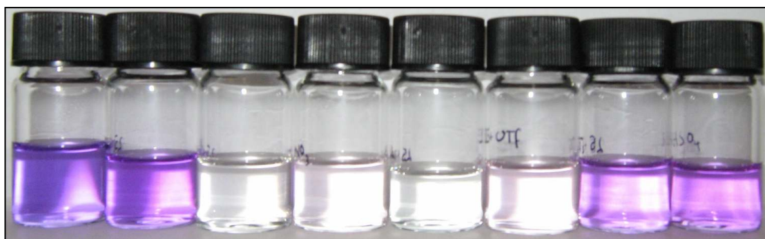
Figure 3.16 – 1 \times 10^{-5} \text{ mol dm}^{-3} solutions of 3.1 at pH 1 in presence of (left to right): \text{Cl}^- ; \text{Br}^- ; \text{I}^- ; \text{NO}_3^- ; \text{OAc}^- ; \text{OTf}^- ; \text{OTs}^- ; \text{HSO}_4^- .
