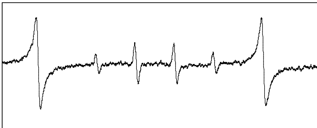
Figure 3.5: A typical example pattern produced by EPR. The Middle four peaks represent \text{OH}\cdot radical release and the large outer two peaks are from the \text{Mn}^{2+} standard.
