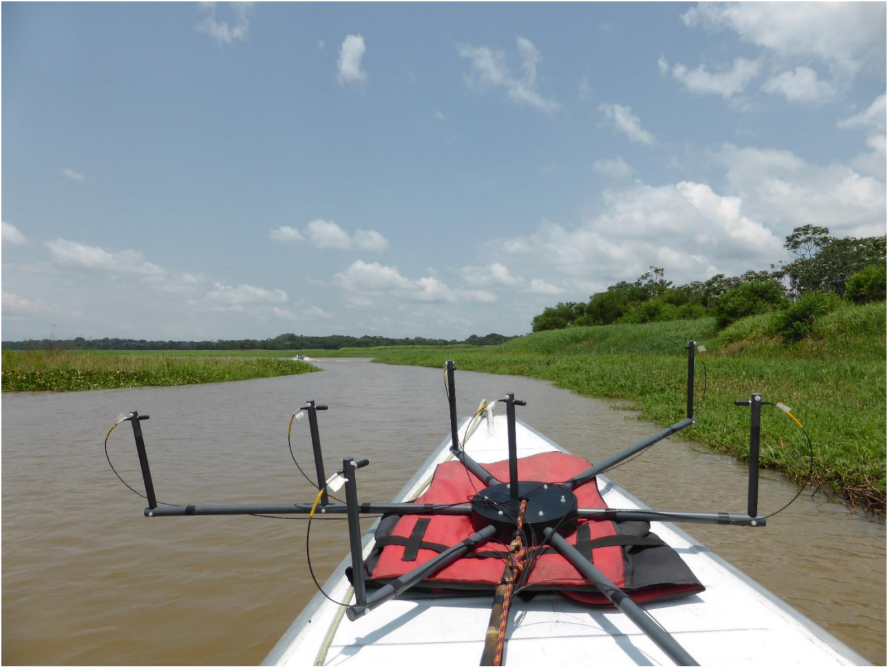
Fig. S1. Photo showing the star array conformation. During trials a GoPro camera was mounted on the wooden stick seen in the bottom of the photo immediately above the black centre disc. Note that one of the TC4013 hydrophones is outside the frame in the bottom right corner. Note also that on the PVC cylinder to the left where two hydrophones are attached only the outermost one was in use during the recordings of this study.
