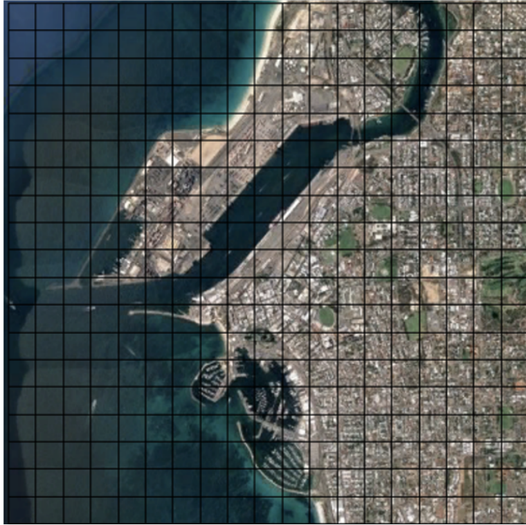
Figure 2.7: High resolution domain over Fremantle inner harbour used to model the location of the exceedance of the NEPM maximum 1 hour average concentration for \text{SO}_2 simulated by AERMOD. The figure shows the location of 400 receptors spaced 250 m apart.
