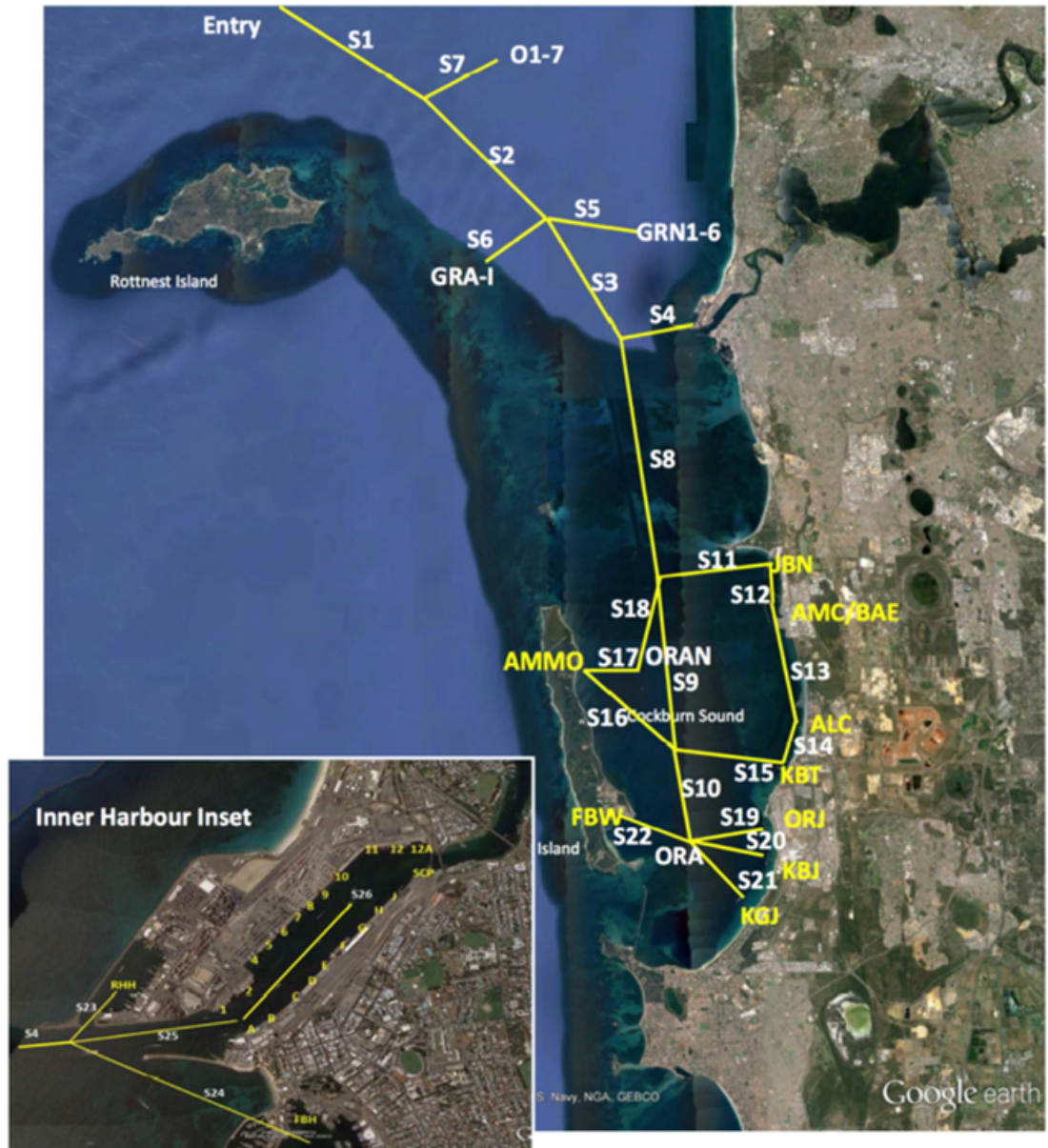
Figure 2.6: Fremantle port berth and anchor locations, and transect segments within port waters. The yellow lines (S1 to S22) denote ship transect routes and remaining locations denote berth and anchor points (Rolfe, 2016).
