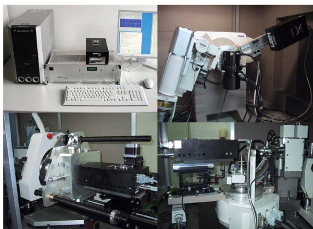
Figure 8. (Color online) Combination of PILATUS 100K (top left: PILATUS 100K system; top right: PILATUS 100K with XRD-DSC II; bottom left: PILATUS 100K with Nano-Viewer; bottom right: PILATUS 100K with AFC-10).
