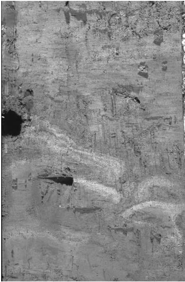
Figure 8. Photograph showing the upper part of event horizon S5 with the deformed silt and silty sand layers at Seewen borehole SR1. The core diameter is 100 mm.
