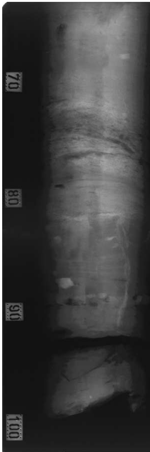
Figure 10. X-ray radiogram showing the trace of the small sand dyke of event horizon S9. The scale is in centimetres.
