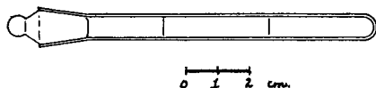
Figure 6. Small stoppered glass tube used for equilibration of n-heptane and salt solutions.
