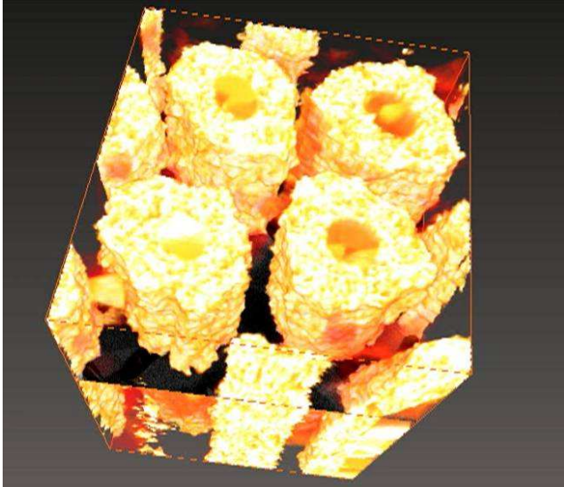
Fig. 1: Nb 3 Sn superconductor filaments: 2048x1536 pixels, 1700 slices (10x10x10nm voxel)
