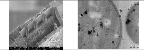
Yeast cells were cryo-fixed in a copper tube by high-pressure freezing and prepared according to the description above. The SE image on the left hand side depicts are row of thinned lamella. On the right hand side a TEM image of the frozen-hydrated yeast cells is shown.
