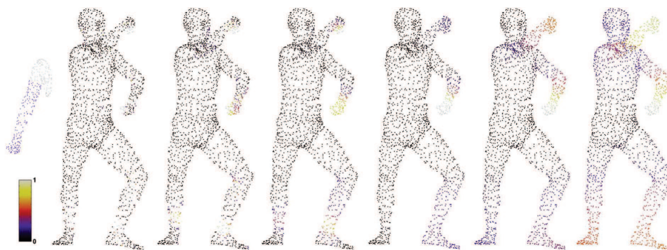
Figure 4: The influence of the parameter \lambda_r , controlling the impact of regularization. The leftmost figure depicts a query part; figures on the right are the membership function u for increasing values of \lambda_r .
