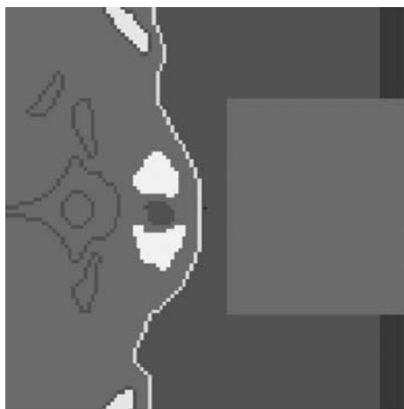
Figure 3. Schematic chart of the position of the detector on the ICRP 100 male phantom. Thyroid glands appear in light colour.
