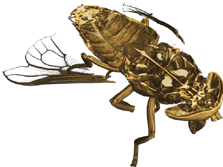
Figure 5: Example from the high resolution neutron tomography: horsefly; length scale about 12 mm, voxel size 13.5 \mu\text{m} ; the high contrast for organic materials can be exploited favourably in this case
