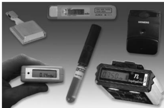
Figure 4. Some personal dosimeters for neutrons or for mixed neutron/photon radiation used within the EVIDOS project.
